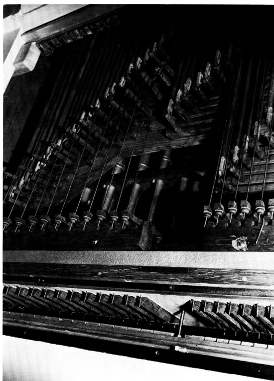
Fig. 152. Udsnit af orglets komplicerede trakturmekanik (s. 164). Annelise Olesen fot. 1975. – Detail of the unusual and complicated tracker action of the organ.
