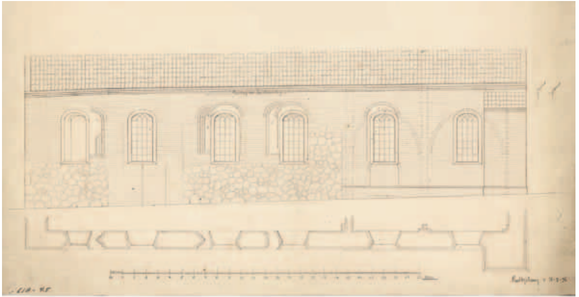
Fig. 16. Kirkens sydmur, plan og opstalt. 1:200. Opmåling, 18. aug. 1896, med registrering af detaljer og ældre åbninger foretaget under restaureringen, formentlig af Hector Estrups konduktør J. Nielsen (s. 1364). I Horsens Museum. – South wall of church, plan and elevation. Scale drawing, 18 August 1896, registering details and older openings made during the restoration, presumably by Hector Estrup's clerk of works, J. Nielsen.
