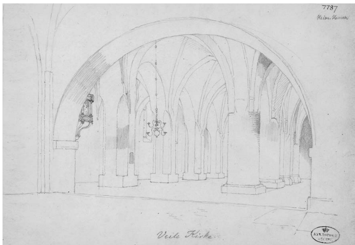
Fig. 11. Skibets indre set mod sydvest fra det gamle \dagger kor, umiddelbart før korets nedbrydning 1855. Den brede \dagger korbue var kommet til 1790-91 ved Anders Kruuses ombygning (s. 106). Af skibets hvælvpillær, der blev ændret og 'uniformeret' ved Carl Lendorf 1862, har de to vestre i nordre række (th.) bevaret deres oprindelige firpas-form (s. 95), mens de to østre i samme række 1630 var ommuret til rundpillær af Peter de Castella (s. 106). Pillærerne i den søndre række (tv.) står i den form, de havde fået ved tilføjelsen af søndre sideskib (s. 101). Tegning ved Heinrich Hansen. – Interior of the nave viewed towards the south west from the old \dagger chancel, just before the demolition of the chancel in 1855. The wide \dagger chancel arch had been added in 1790-91 in Anders Kruuse's rebuilding. Of the vaulting pillars of the nave, which were changed and 'uniformized' by Carl Lendorf in 1862, the two western ones in the northern row (right) have kept their original quatrefoil form, while the two eastern ones in the same row were rebuilt as round pillars in 1630 by Peter de Castella. The pillars in the south row (left) stand with the form they had been given with the addition of the south side aisle.
